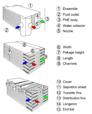
Fig. 5. Installation of the plate heat exchanger made of aluminum
