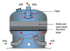
Fig. 2. Container with horizontal layers
