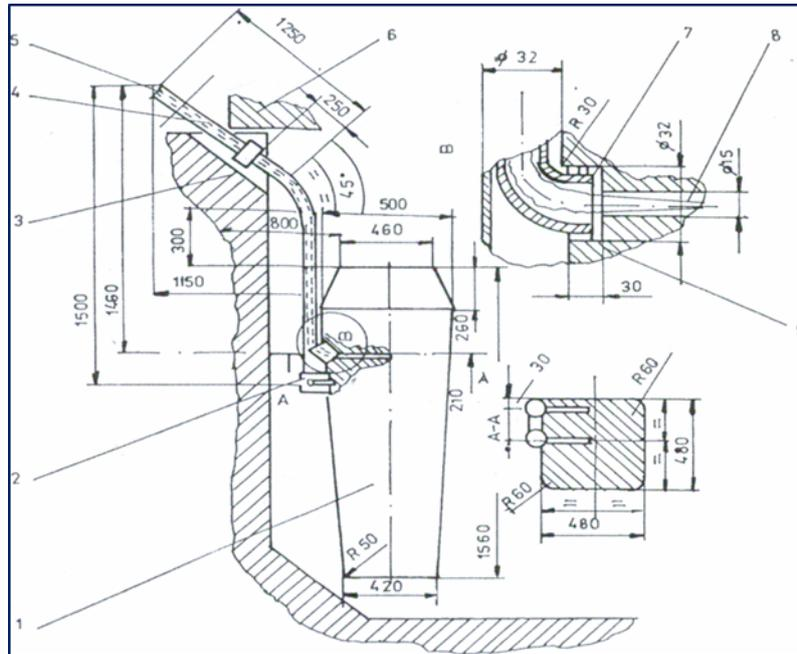
Figure 1. Installing of thermal torques for measurement of the ingot's temperature
